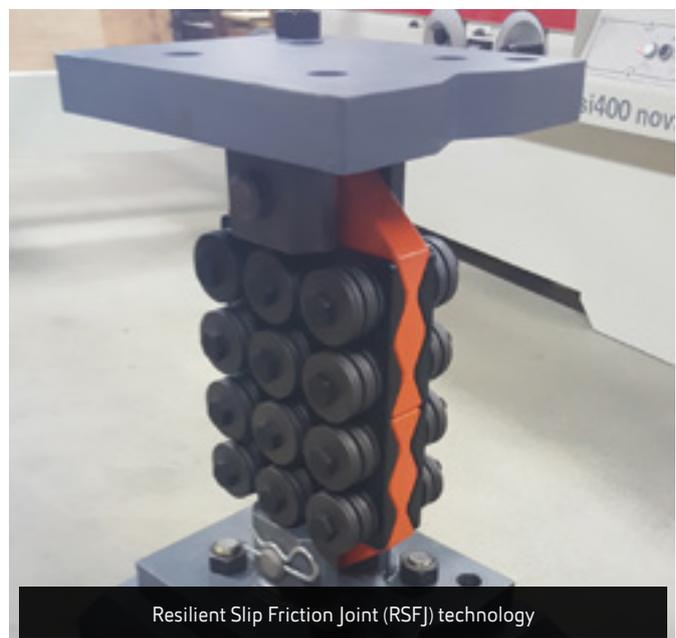
Resilient Slip Friction Joint (RSFJ) technology
