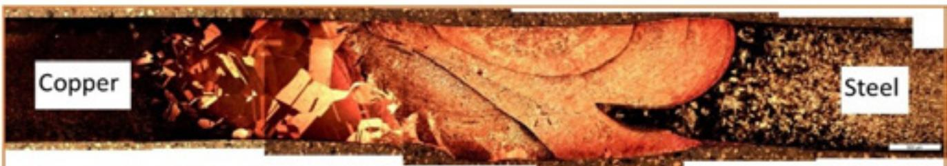
Top left: electron beam welded titanium. Top right: laser welded and TIG welded titanium. Bottom: dissimilar welded copper-steel
