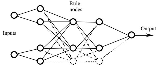
**Figure 3** A FuNN structure of 2 inputs (input variables), 2 fuzzy linguistic terms for each variable (2 membership functions). The number of the rule (case) nodes can vary. Two output membership functions are used for the output variable.
