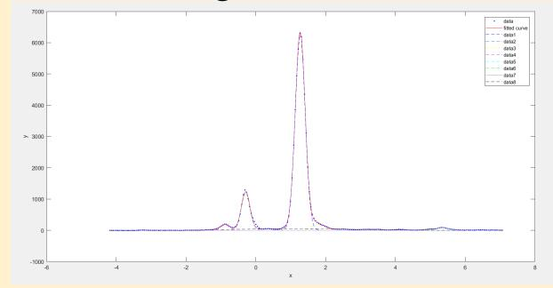
The above plot was made using Matlab's 'fit' function and it features eight Gaussians that have been formulated to approximate the spectral lines of the methanol maser source. The main spectral feature is represented by the sharpest peak, which corresponds to methanol.
