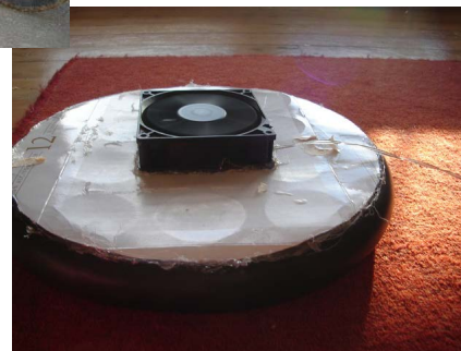
Right - Hovercraft - using computer fan and pram wheel.
