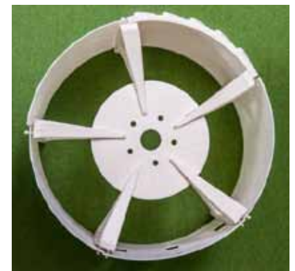
3D printed Mars Rover wheel created as part of the NASA Space Apps Challenge
